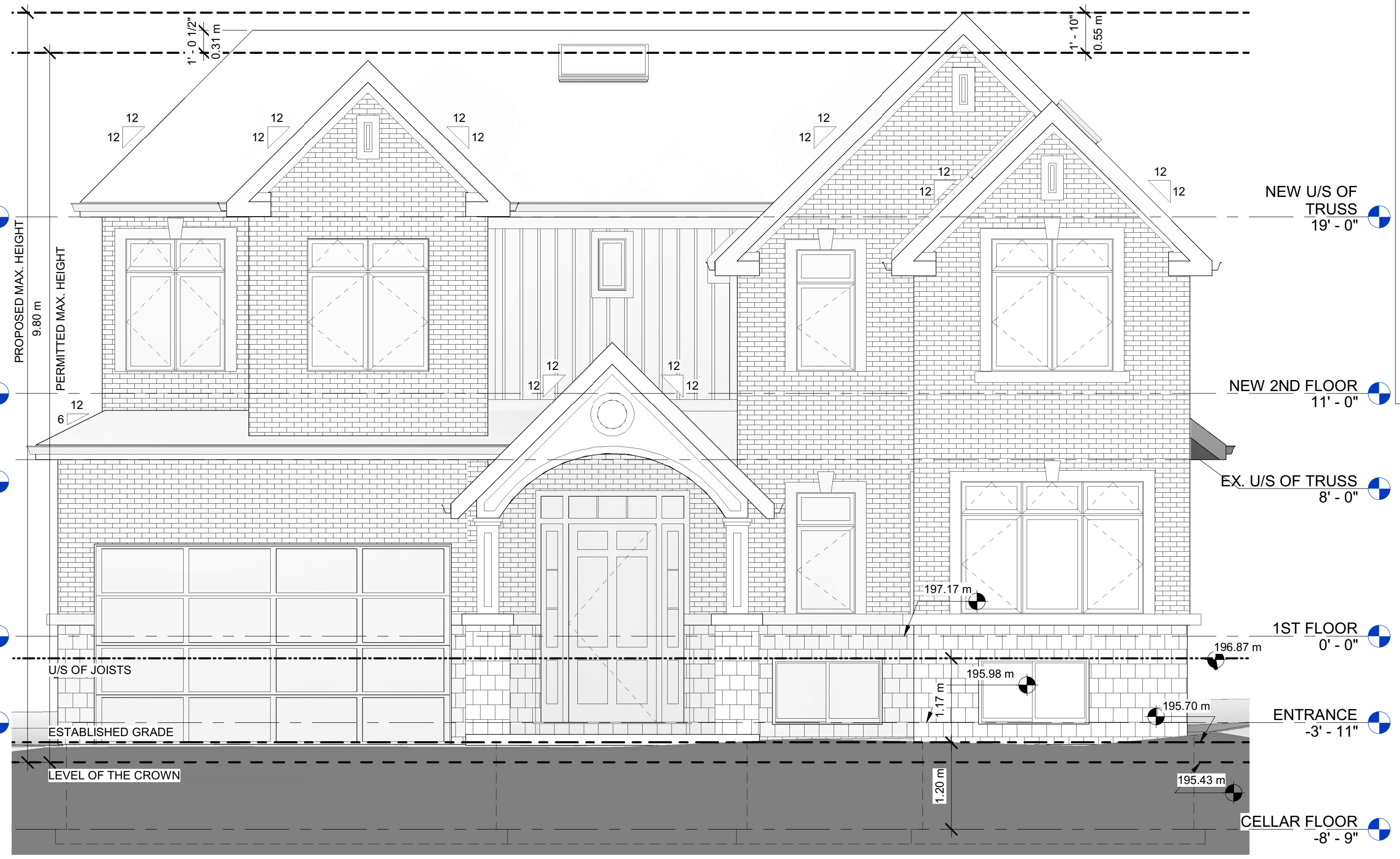
1 NORTH ELEVATION (FRONT) 1/4" = 1'-0"
