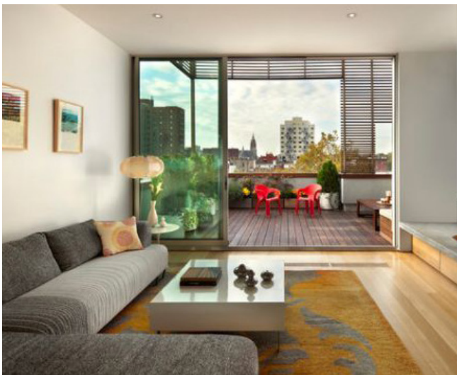
Figure 106. This unit provides a roll-out, no-lip access to the outdoor space accessed directly from the living room.
