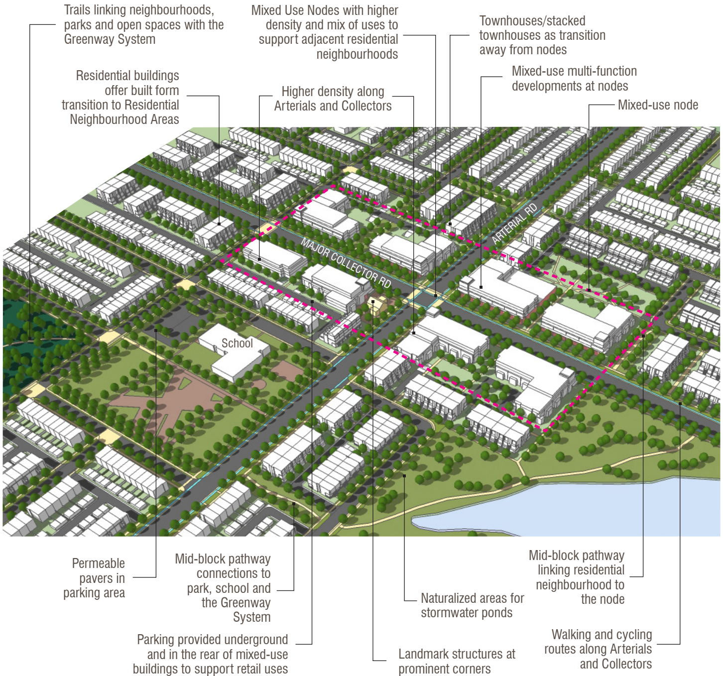
Figure 2.2 Demonstration plan illustrating key organizing elements and built form vision for Mixed Use Neighbourhood Corridors and Nodes
