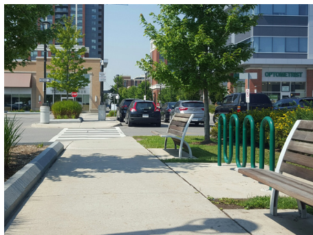
Landscaped islands defining parking courts and clearly identified pedestrian routes
