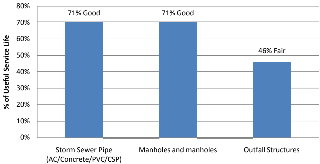
Figure 3-17 % Useful Life By Component and Condition Rating by Age – Stormwater within ROW
