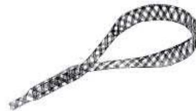
The expansion of the cobra hollow braid rope can be seen clearly. After girdling, the end is inserted into the outgoing rope by stretching the meshes. This connection type is called Quick Splice. To avoid chafing of rope the girdling area is wrapped in a polypropylene friction sleeve tube.
