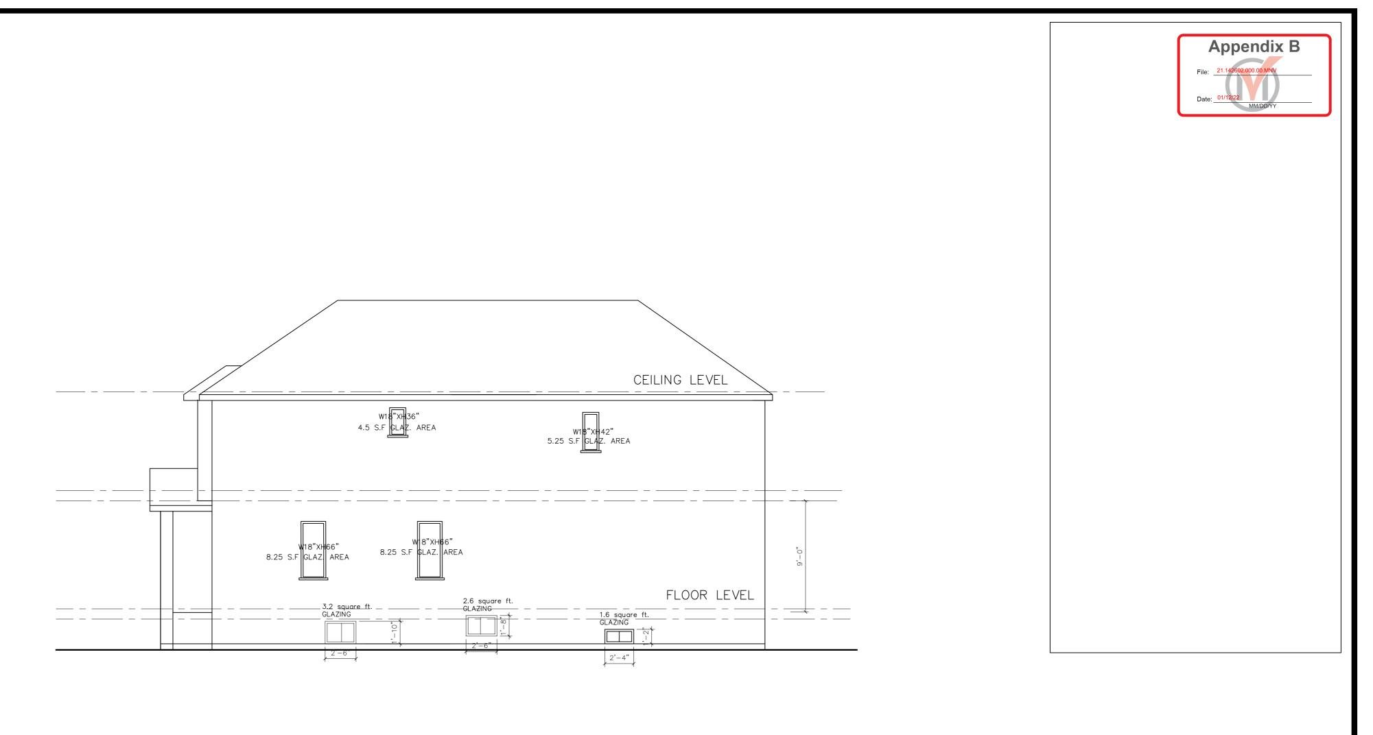
Table 9.10.15.4. Maximum Area of Glazed Openings in Exterior Walls of Houses 7.0% MAX.window openings
