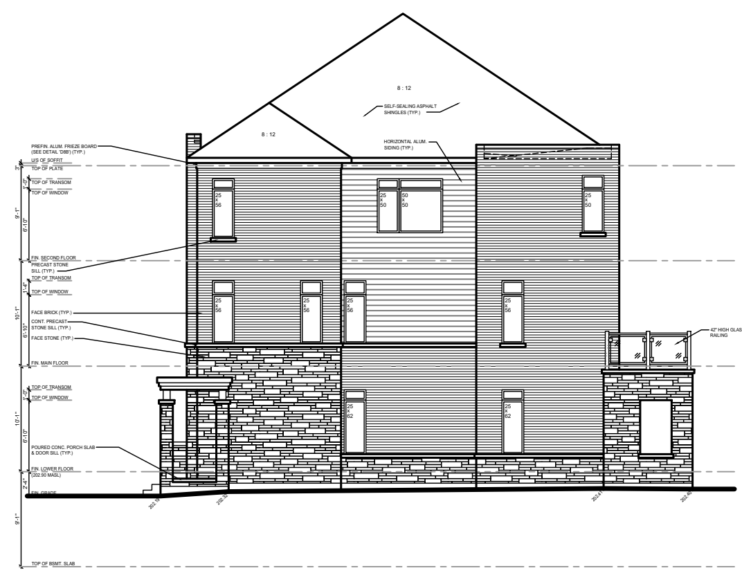
BLOCK A LEFT SIDE ELEVATION
