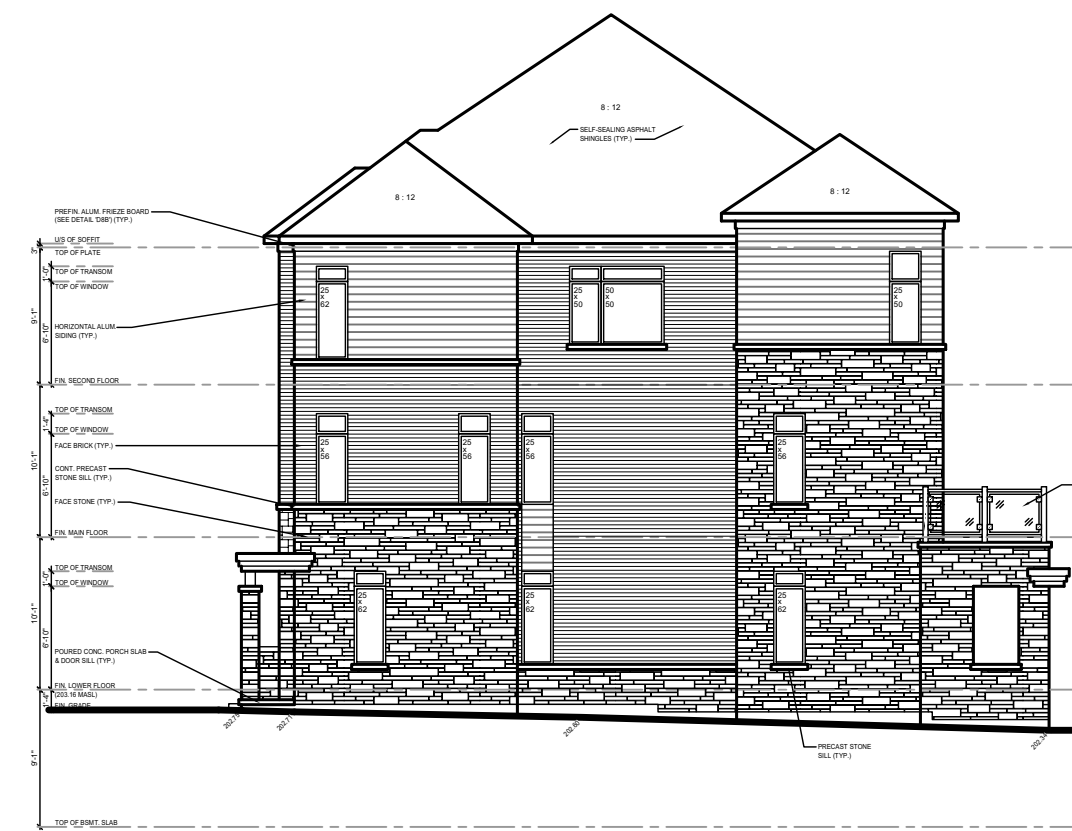
BLOCK J LEFT SIDE ELEVATION
