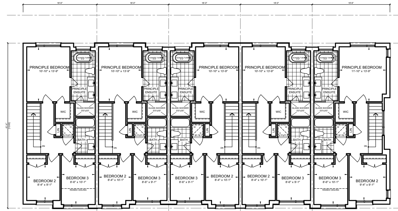
BLOCK A SECOND FLOOR PLAN
