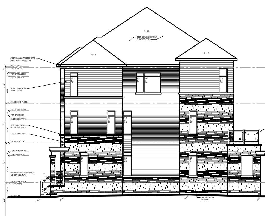
BLOCK K LEFT SIDE ELEVATION
