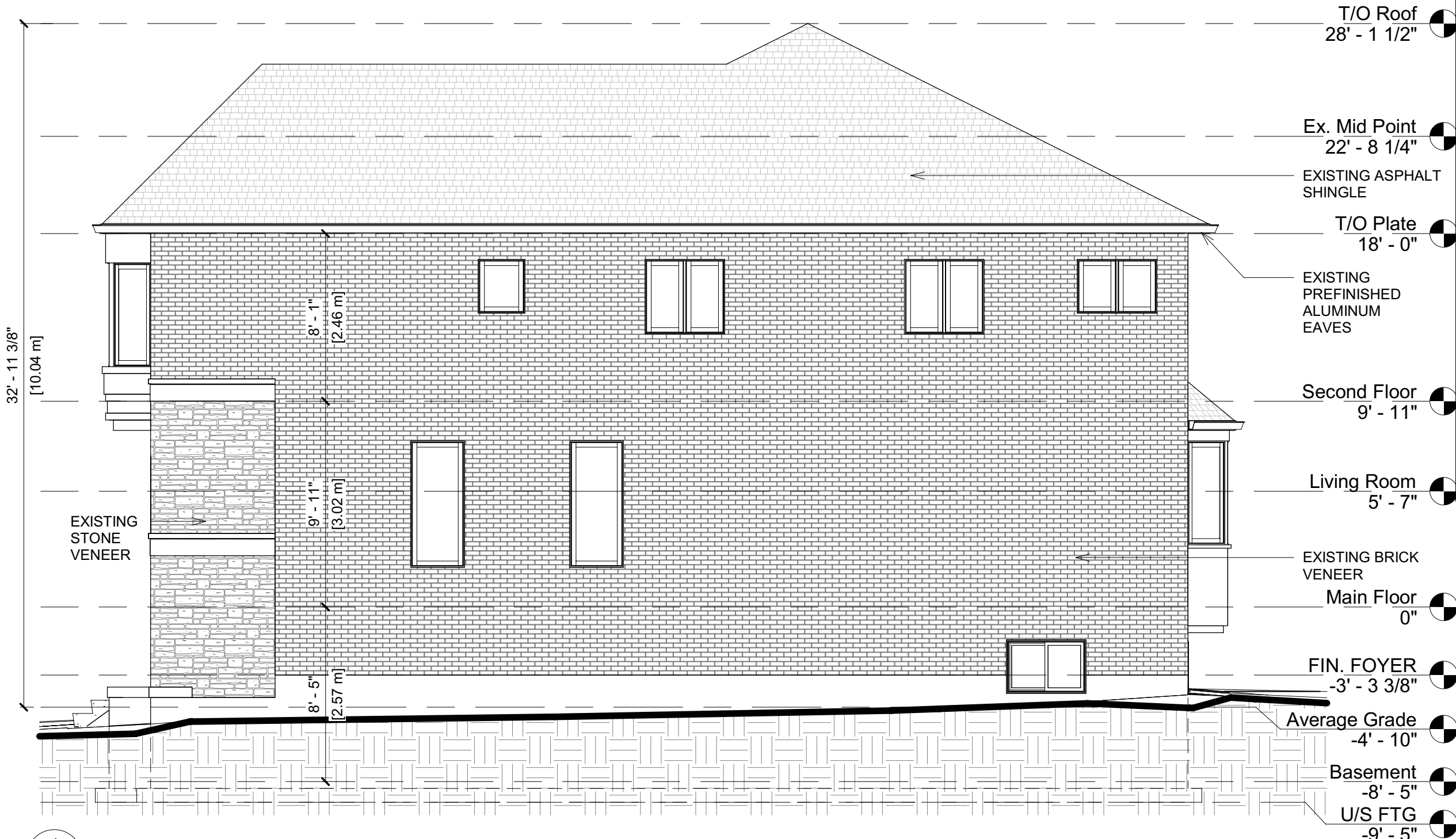
1 EXISTING WEST ELEVATION A2.04 3/16" = 1'-0"
