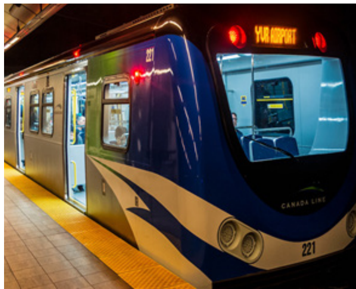
Figure 3. Hyundai Rotem Light Rail Transit – Canada Line Two Car Trainsets – 168,000 passengers a day Canada Line – Electric, Driverless, Automatic Train Control, 2 car trainsets Line Length – 19km, 16 Stations and 3 more Stations to be added Platform Length – 11 - 40 metre long, 5 stns-50 meters & 3 more 50m Stns Daily Ridership – 168,000 passengers going to 235,000 ridership. Frequency – Peak Hours 2 minutes – non-Peak - 5 minutes 2 Car trainset, seating 88 passenger, crush load capacity 400 passengers Driverless, automatic train control and powered by 750 V DC Canada Line Stations – All planned as Complete Destinations TOD stations. If the Canada Line stations were to be enlarge the 11 40-meter train station platforms would be enlarged to 50 meters, they will be able to add one more passenger car and increase daily ridership to 350,000 passengers at day.
