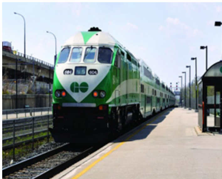
Figure 2. Bombardier Diesel Locomotive (Heavy Rail) Stouffville Line - 12 Car Double Decker Trainsets – 18,500 passenger a day Stouffville GO Transit Line – Diesel Locomotive, 12 double-decker cars Future Electrification – 25,000 V AC. Line Length 48km, Platform Length – 300 meters long Daily Ridership - 18,500 passengers. Currently 11 stations at 300 metre long and 5 more 300 metre stations have been approved but not built Peak -15 minutes, non-Peak 60 minutes Train Capacity – 12 double decker passenger cars Seating Capacity –1200-1800 passengers per trip –12 double decker cars Crushed numbers – 3600 passengers per 12 car train Nearly all Stouffville GO Line Stations are parking lots. Lincolnville to Union Station – 1 hr and 3 mins – 11 station stops. Add 5 Stns - Lincolnville to Union Station daily commute - 1hr & 23 mins
