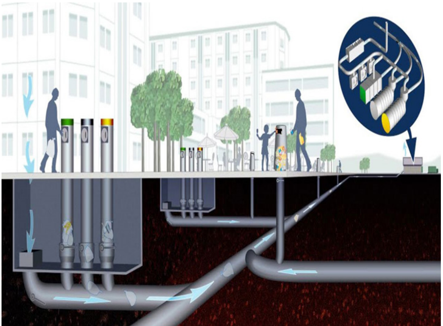
Figure 15. High-Speed Powered Chute Systems For Waste Removal
