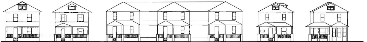
3. Appropriate: the Building scale is reduced through articulation of the existing building facade. Rhythm, alignment and spacing are based on the existing context.
