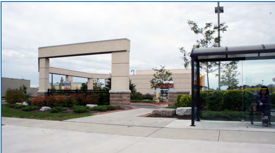
Figure 4.7g: This gas bar and drive-through facility at Bur Oak Avenue & McCowan Road utilizes an architectural screen to buffer the stacking lane from the street while maintaining a built form edge along the street.
