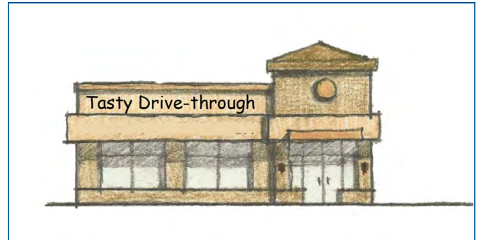
Figure 4.7c: Sketch of the facade of a drive-through facility which provides appropriate fenestration and entrance features.
