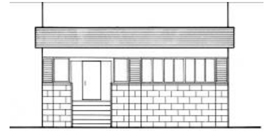
Porch filled in, inconsistent with character of the building..
