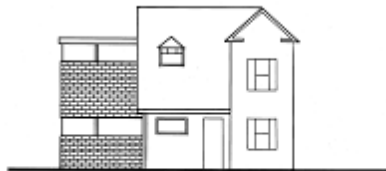
Incompatible contrast: addition is too contrasting; draws attention; compromises integrity of original building.
