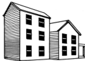
Not Appropriate: scale of addition overwhelms original house
