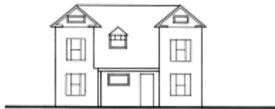
Too Similar: inappropriate scale—compromises composition by confusing the design of the original building.
